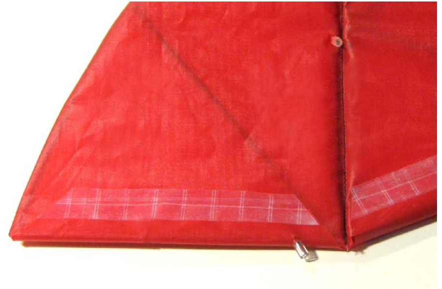
Bottom view showing strut and rear fuselage attachments.
